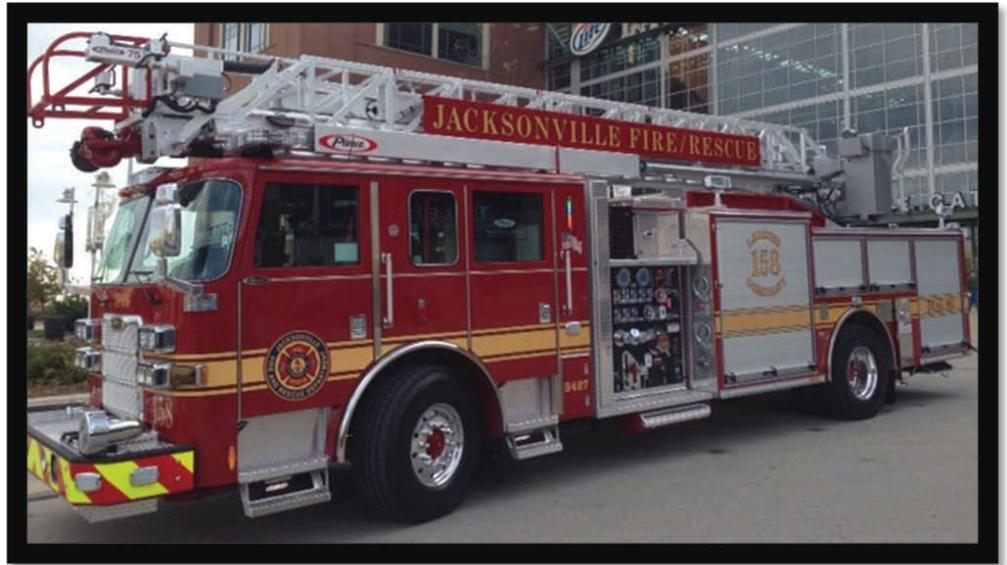
The quint will be officially designated as “Ladder 158”. It will be staffed with four firefighters and feature a 450HP Cummings diesel engine, a 500-gallon water tank, a pump capable of delivering 1,500 gallons of water per minute, and a 75-foot aerial ladder with a waterway for elevated fire suppression. It will be equipped with extrication tools as well as being licensed as an Advanced Life Support apparatus.
